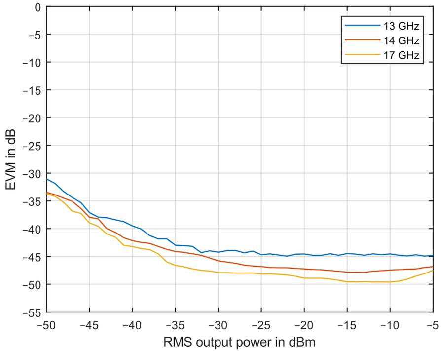
Measured EVM of a 2 GHz 5G NR signal, full allocation, SCS: 960 kHz, modulation: 256QAM, optimize EVM turned on, using the R&S®FSW signal and spectrum analyzer with the R&S®FSW-K575 I/Q noise cancellation option (IQNC with 50 iterations)
