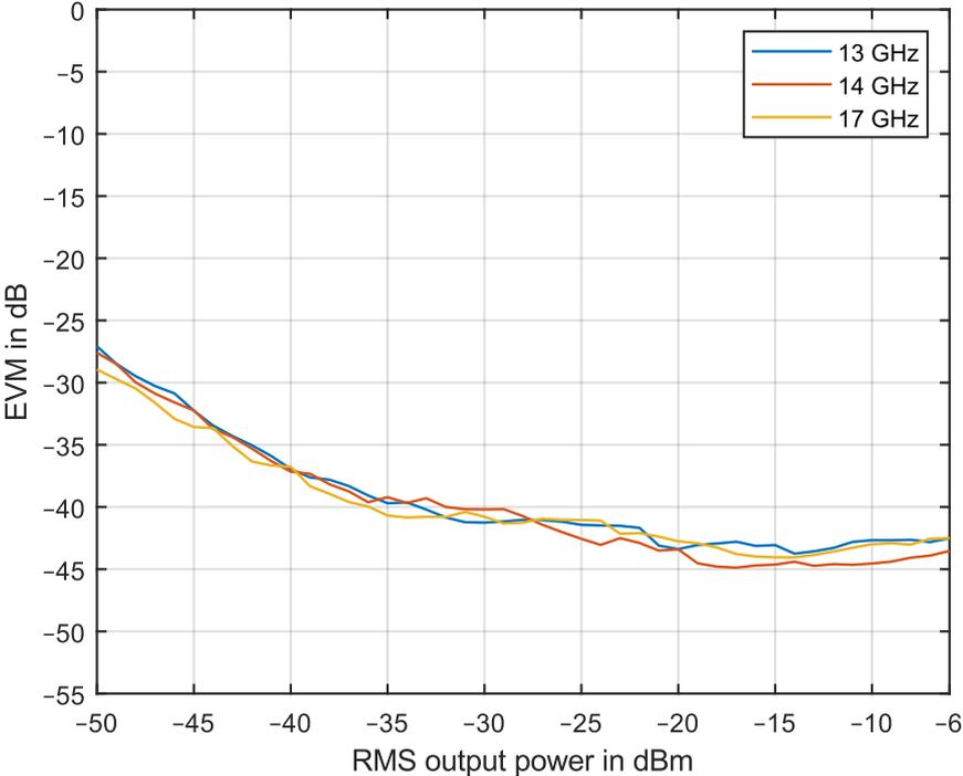
Measured EVM of a 4 GHz OFDM signal, full allocation, SCS: 960 kHz, modulation: QPSK, optimize EVM turned on, using the R&S®FSW signal and spectrum analyzer with the R&S®FSW-K575 I/Q noise cancellation option (IQNC with 50 iterations)
