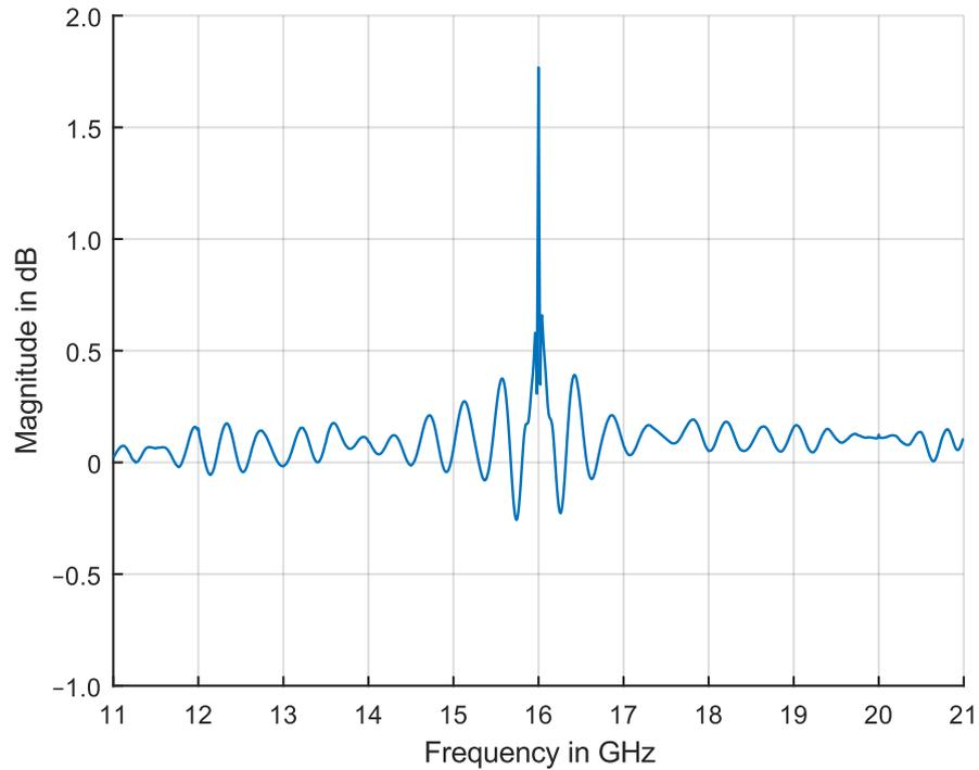
Measured frequency response, level = 0 dBm, RF output
