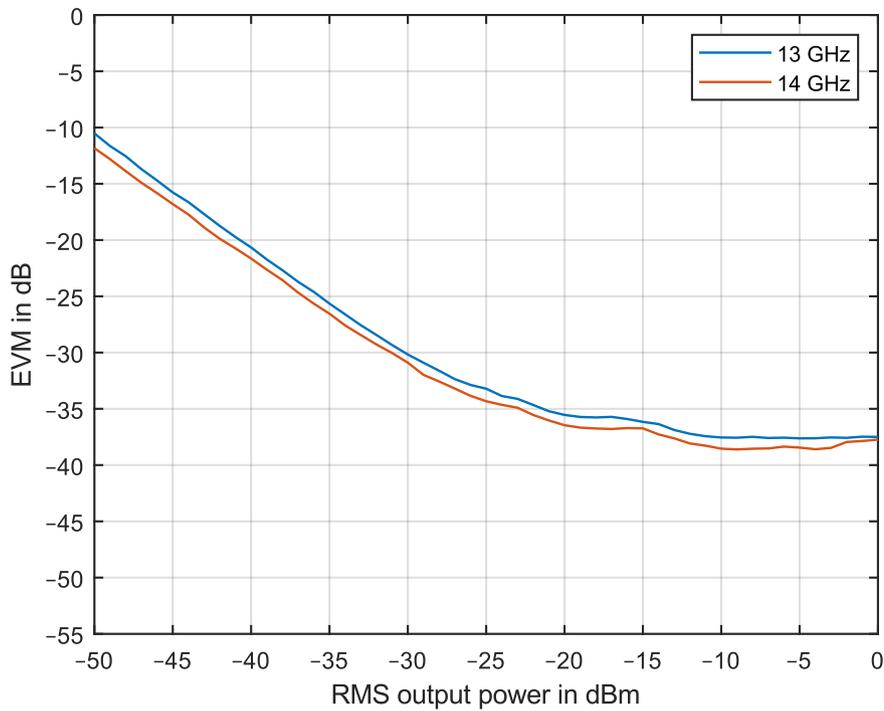
Measured EVM of a 4.32 GHz IEEE 802.11ay EDMG signal, NCB2, modulation: 16QAM, optimize EVM turned on, using the R&S®FSW signal and spectrum analyzer
