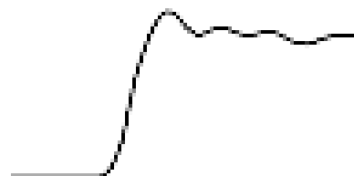
Figure 7: Signal with a long ground lead
