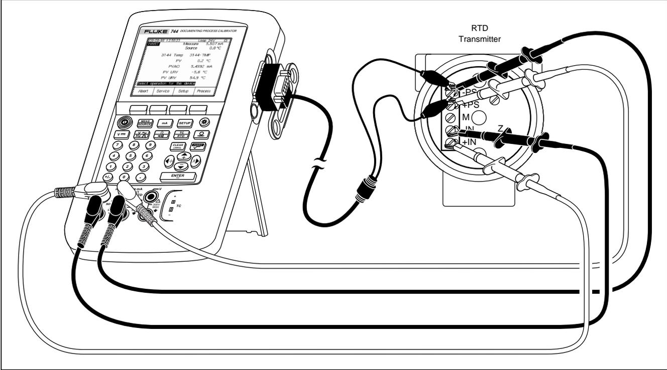
**Figure 1. Connecting to a HART Transmitter**
