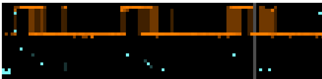
Figure 7-4: Unipolar PWM signal with duty cycle track M1, which is the demodulated waveform
