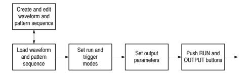
Figure 3-5: Waveform output sequence example
