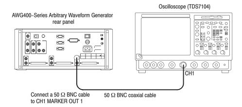
Figure B-40: Marker output initial test hookup
