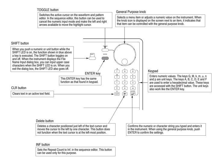
Figure 2-2: Front panel keypad area
