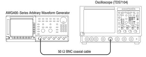
Figure B-20: Direct DA output pulse rise time initial test hookup
