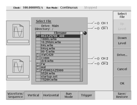
Figure 2–28: Setup Waveform/Sequence menu
