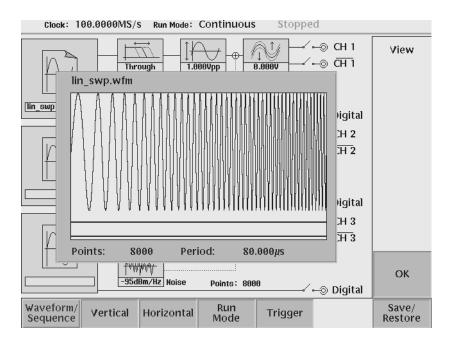
Figure 2–37: Viewing a waveform loaded into memory
