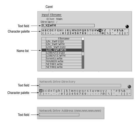
Figure 2–12: Three type of Input text dialog boxes
