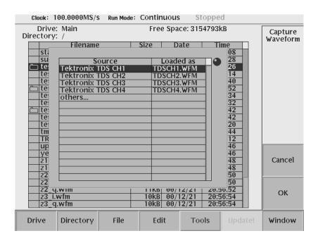
Figure 3-77: Source instrument selection dialog box
