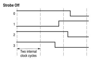
The instrument reads this state in an unstable transition period. This may cause an erroneous action.
