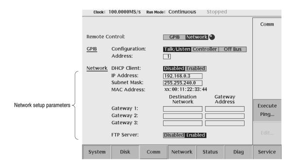
Figure 3-68: Network setup screen menu
