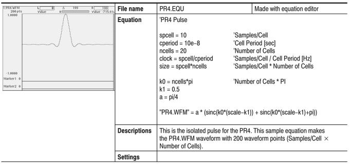
Table D-16: Isolated pulse for disk application (EPR4.EQU)
