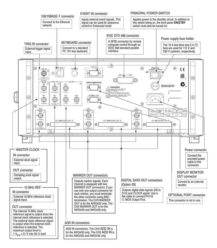
Figure 2-4: Rear panel signal and power connectors
