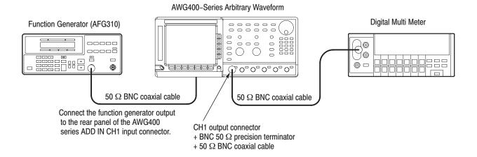
Figure B-39: ADD IN input initial test hookup
