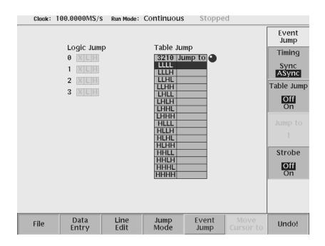
Figure 2-51: Screen for setting jump mode
