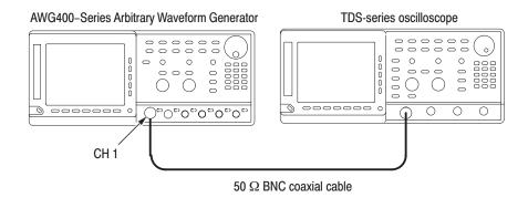
Figure 2–33: Cable connection between AWG400-Series Arbitrary Waveform Generator and digital storage oscilloscope
