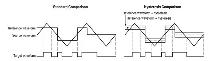
Figure 3-11: Waveform compare operation example
