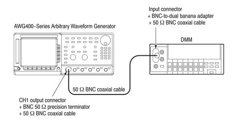
Figure B-15: Amplitude accuracy initial test hookup
