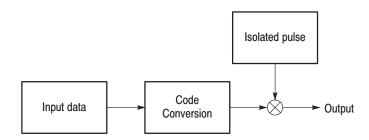
Figure 3-37: Outline flow for producing network test read signal
