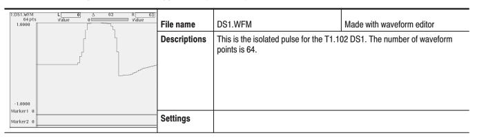
Table D-20: Isolated pulse for network application (DS1A.WFM)
