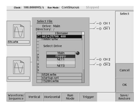
Figure B-5: Loading file; selecting storage drive
