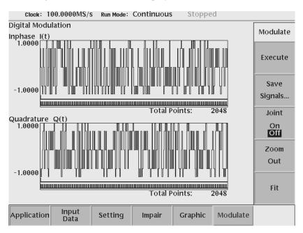
Figure 3-55: Execution of digital modulation
