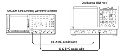
Figure B-42: Channel skew test hookup
