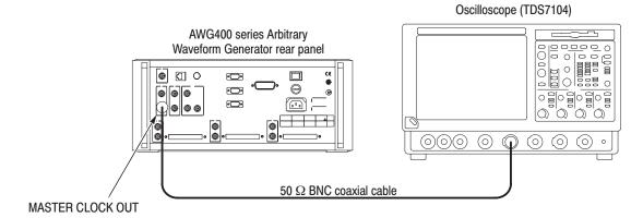
Figure B-43: Master Clock output initial test hookup
