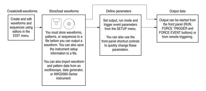
Figure 3-1: Overview of AWG400-Series Arbitrary Waveform Generator process flow
