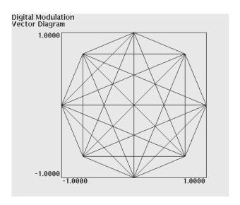
Figure 3-62: Vector diagram display screen
