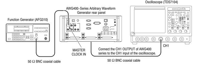
Figure B-38: Master Clock input initial test hookup
