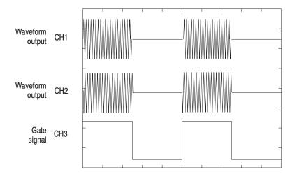
Figure B-12: Relationship between gate signal and waveform output (Instrument other than option 05)
