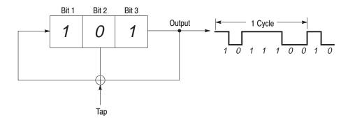
Figure 3-8: Register value and tap setting example
