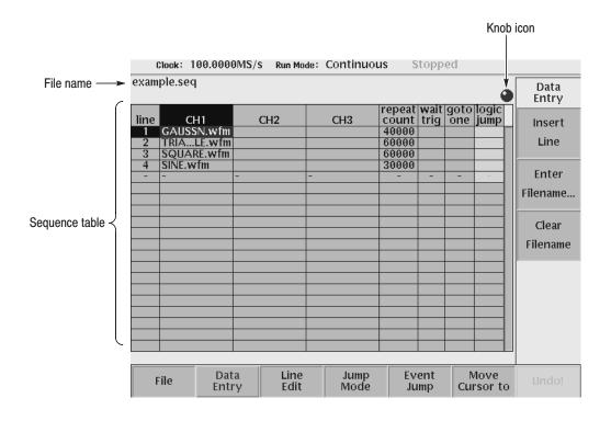
Figure 3-28: Sequence editor screen with example sequence list
