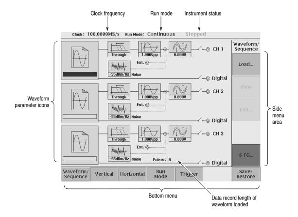
Figure 3-3: Main Setup screen (AWG430)
