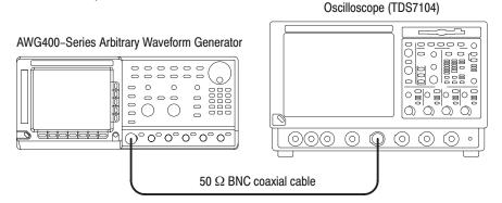
Figure B-21: Step response initial test hookup
