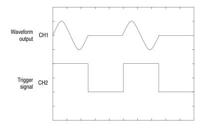
Figure B-11: Relationship between trigger signal and waveform output (Instrument with option 05)
