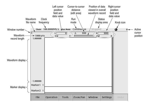
Figure 3-6: Waveform editor initial screen
