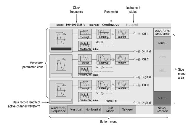
Figure 3-2: Setup main screen
