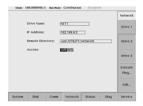
Figure 3-71: UTILITY screen mounting remote file system
