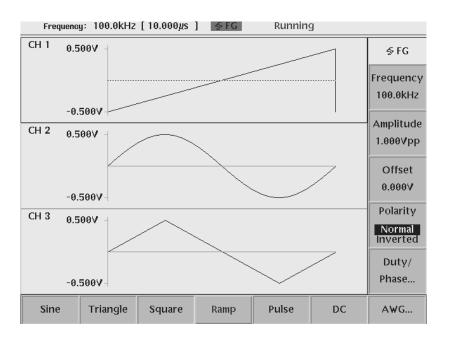
Figure 3-92: FG mode screen (AWG430)
