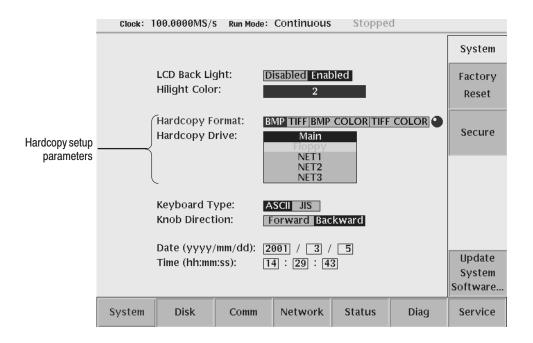
Figure 3–73: Hardcopy setup screen
