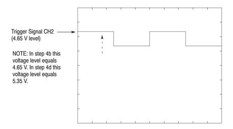
Figure B-25: Trigger Signal (+5V check1)
