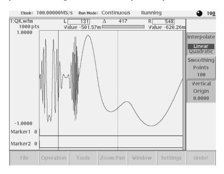
Figure 3-22: A waveform example under quick editing
