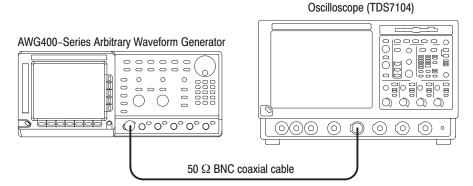
Figure B-19: Direct DA output pulse rise time initial test hookup
