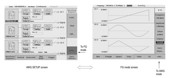
Figure 3–93: Change the generator mode (AWG430)
