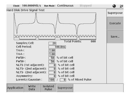
Figure 3-36: Execution of superpose
