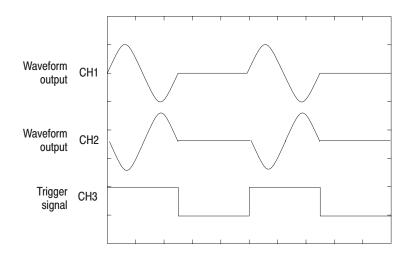
Figure B-9: Relationship between trigger signal and waveform output (Instrument other than option 05)
