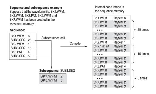
Figure 3-31: Compiling and storing sequences and subsequences
