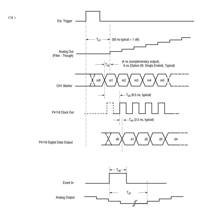
Figure A-3: Signal timing
