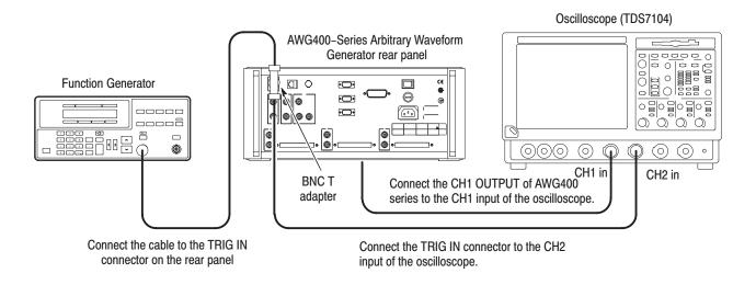
Figure B-24: Trigger input initial test hookup
