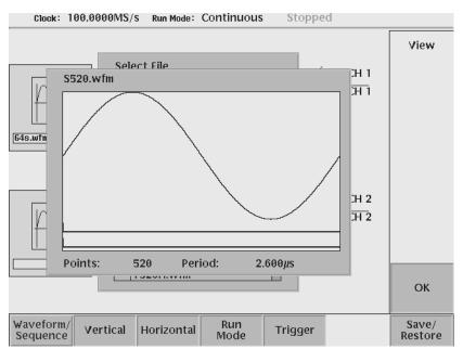
Figure 2-21: Viewing a file by Quick View function
