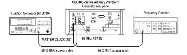
Figure B-37: 10 MHz reference input initial test hookup
