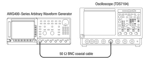
Figure B-22: Step response initial test hookup
