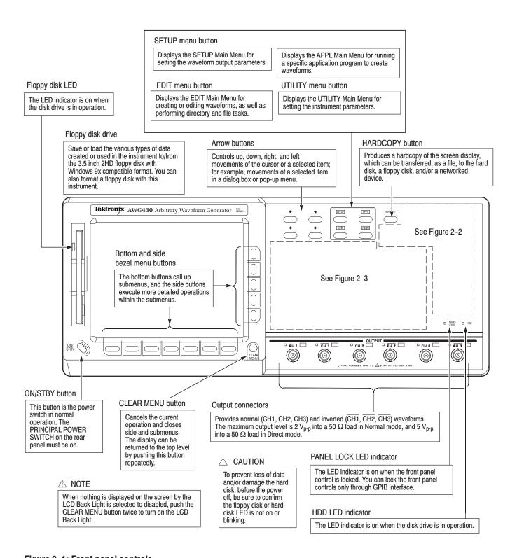
Figure 2–1: Front panel controls
