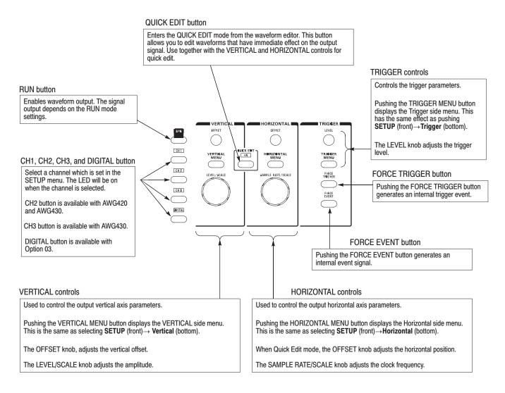
Figure 2-3: Front panel keypad area
