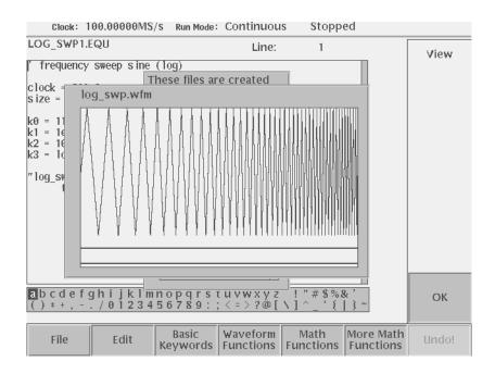
Figure 2-47: Viewer displaying compiled waveform
