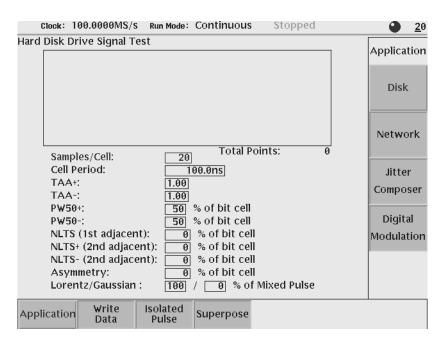
Figure 3-33: Disk application initial screen
