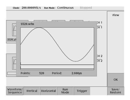
Figure 2-29: Viewing a file in the Setup screen
