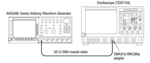
Figure B-23: Internal trigger initial test hookup
