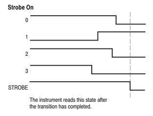
Figure 3-30: Event signal timing and strobe
