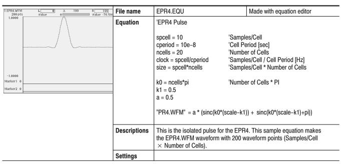
Table D-17: Isolated pulse for disk application (E2PR4.EQU)
