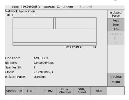
Figure 3-40: Side menu for selecting the Isolated pulse
