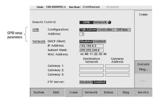
Figure 3-67: GPIB setup screen menu
