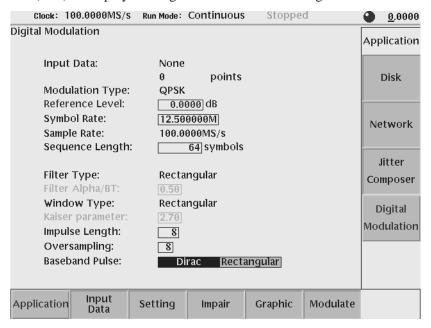
Figure 3-50: Digital Modulation application initial screen
