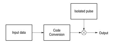
Figure 3-32: Outline flow for producing HDD reading test signal
