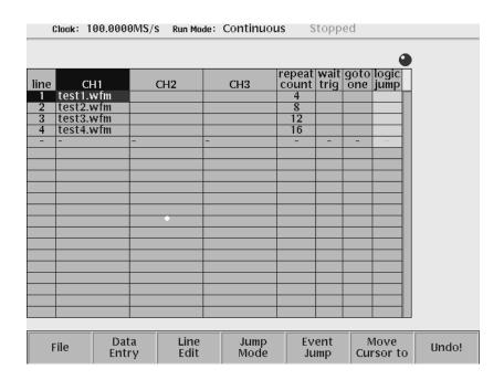
Figure 3-82: Sequence generated by the Example 3 equation
