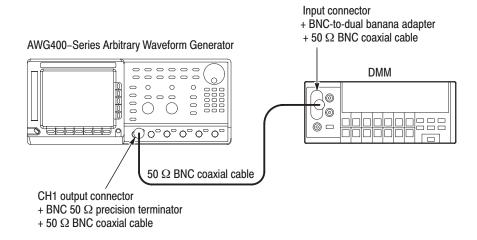
Figure B-17: Direct DA output amplitude accuracy initial test hookup
