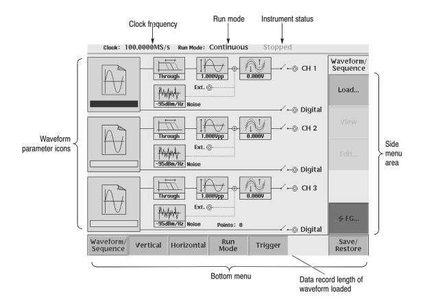
Figure 2-27: Main Setup screen (AWG430)
