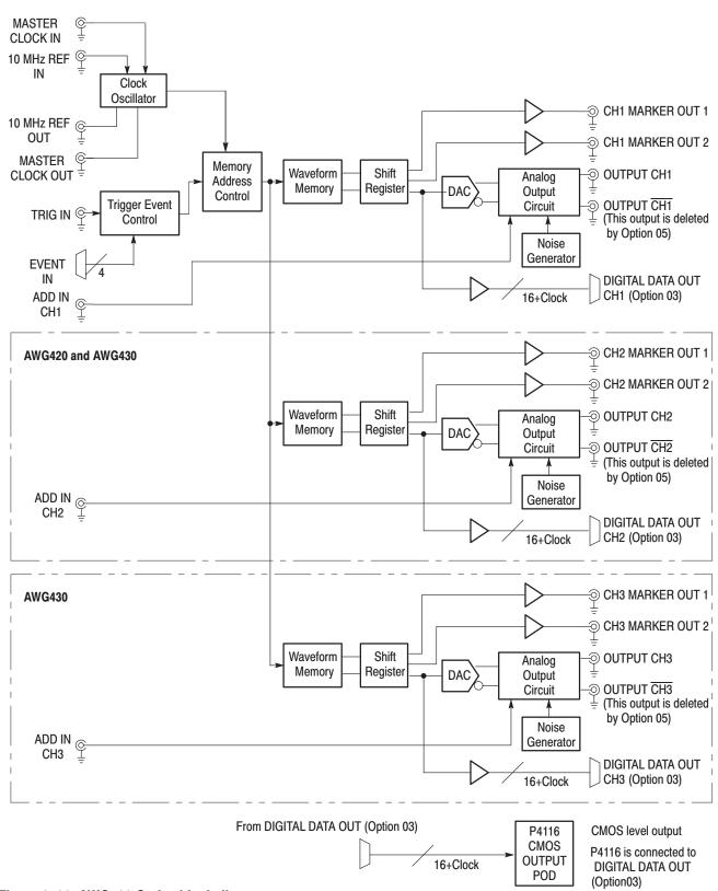
Figure 2-30: AWG400-Series block diagram
