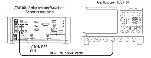
Figure B-44: 10MHz Reference output initial test hookup
