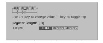
Figure 3-9: Shift Register Generator dialog box
