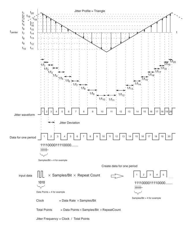
Figure 3-48: Jitter parameters and jitter waveform
