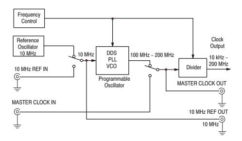
Figure 2–31: Clock oscillator configuration.
