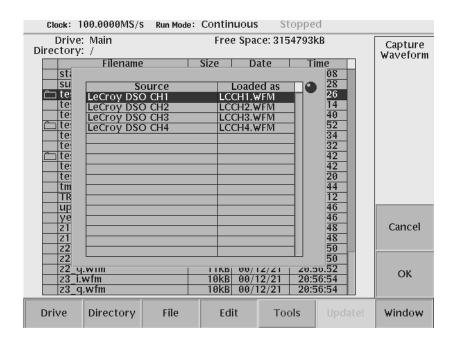
Figure 3–78: Source instrument selection under Others...
