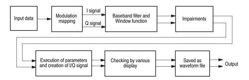
Figure 3-49: Outline flow for producing digital modulation waveform
