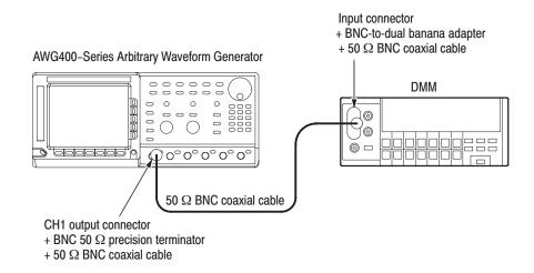
Figure B-16: Amplitude accuracy initial test hookup
