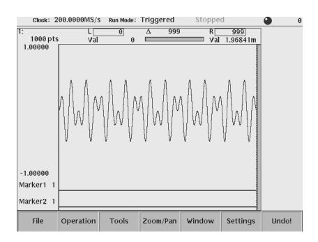
Figure 2–42: Waveform created with the multiply operation
