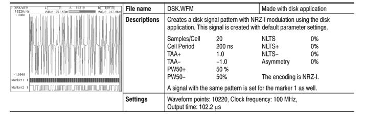
Table D-15: Isolated pulse for disk application (PR4.EQU)
