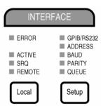
[Setup] Pressing the [Setup] key cycles through GPIB/RS-232, ADDRESS, BAUD, PARITY and QUEUE. In each case, the appropriate parameter is displayed in the Reference display and the knob is used for adjustment. Press [Phase], [Freq], [Ampl], [Harm#] or [Aux Out] to return the display to normal and leave Setup.
