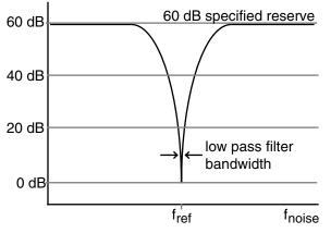
The above graph shows the actual reserve vs the frequency of the noise. In some instruments, the signal input attenuates frequencies far outside the lock-in's operating range ( $f_{noise}$ >>100 kHz). In these cases, the reserve can be higher at these
