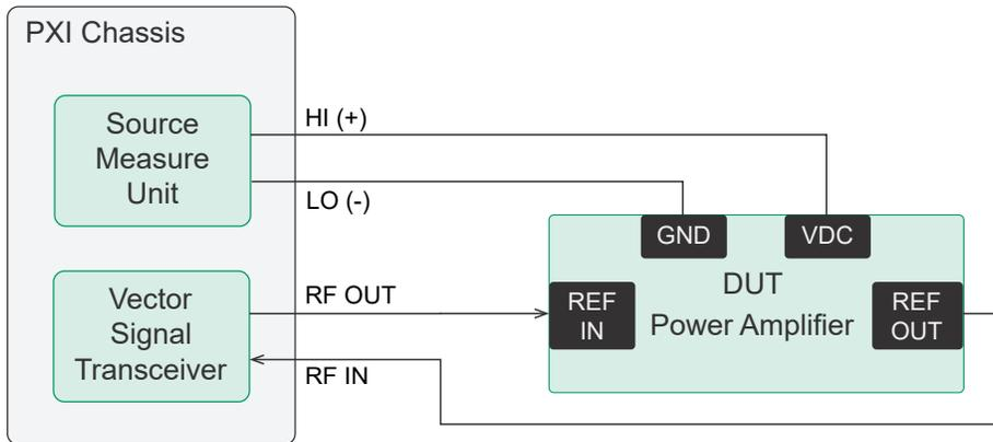
A VST is a combination of a one-port generator and a one-port analyzer with an onboard FPGA. A VST can simultaneously generate a stimulus and receive back the response from the coupled port with minimal phase noise impact due to the LO sharing capabilities between the transmission and receiving path.
