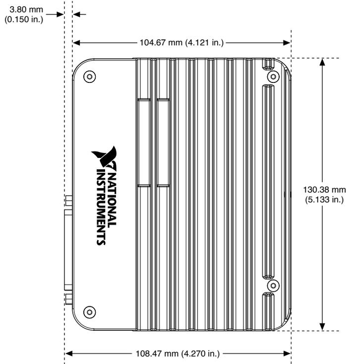
Figure 23. Bottom View with Dimensions in inches [millimeters]
