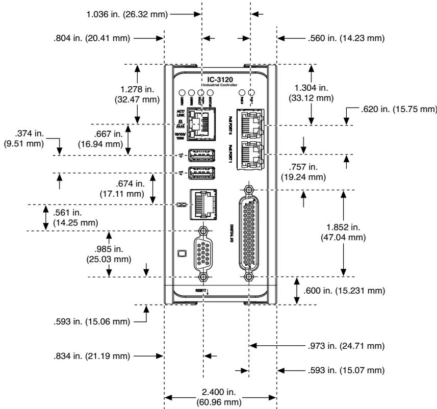
Figure 21. Back View with Dimensions in inches [millimeters]
