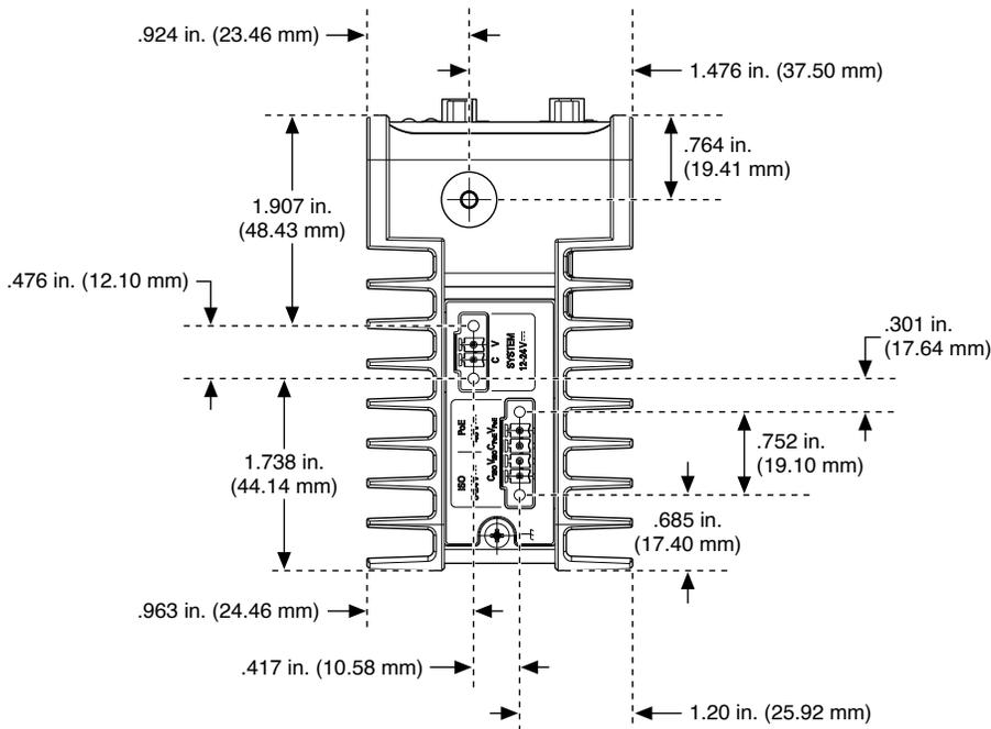
Figure 22. Side View with Dimensions in inches [millimeters]
