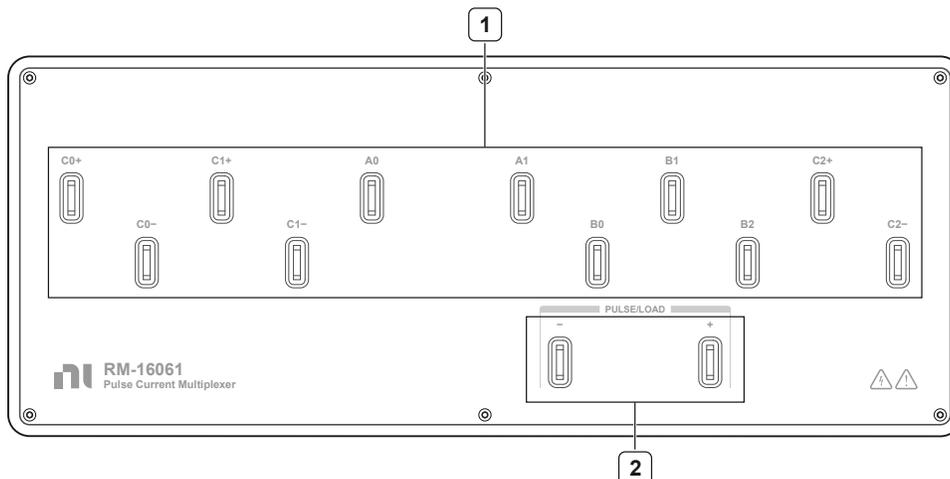
Figure 27. Pulser Connectivity: Human-Machine Interface Side
