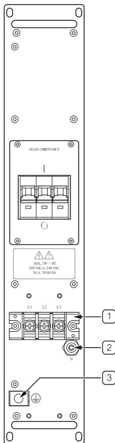
1. M6 screw thread input terminal block
