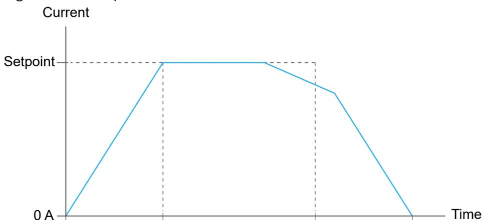
To correct incomplete pulse waveforms, increase the charge voltage.
