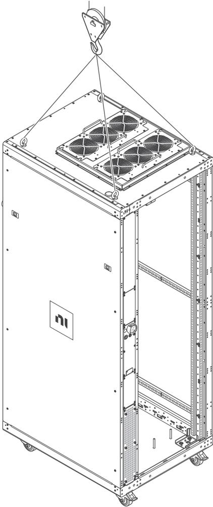
1. Connect the four eyebolts to the mounting holes on the top of the rack.
