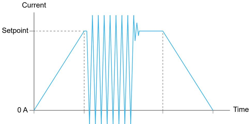
To correct ringing pulse waveforms, decrease the charge voltage.
