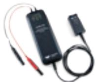
Low cost active differential probes are intended for measuring higher voltages. The differential techniques employed permit measurements to be taken at two points in a circuit without reference to the ground, allowing the oscilloscope to be safely grounded without the use of opto-isolators or isolating transformers.
